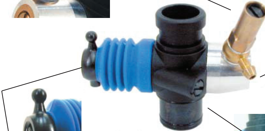
LOW END NEEDLE FACTORY SETTING: HEAD IS FLUSH WITH BALL COLLAR SET: 1/2 TURNS OUT FUNCTION: ADJUSTS THROTTLE RESPONSE.
