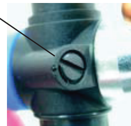
BARREL STOP OR IDLE SCREW FACTORY SETTING: 1/16 AIR GAP
